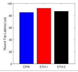
Figure 5. Concurrent CPRI and Ethernet services over 8 km fiber.
