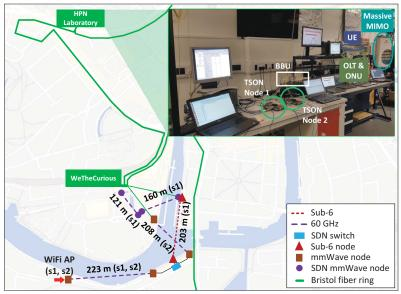
Figure 3. 5G-XHaul BiO testbed overview. Wireless SDN and optical network at HPN laboratory.
