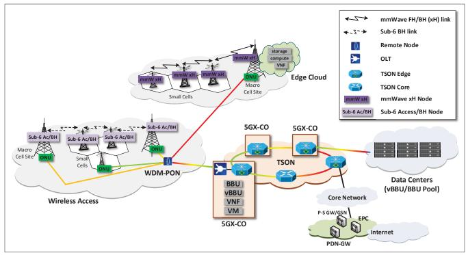
Figure 1. 5G-XHaul data plane architecture.
