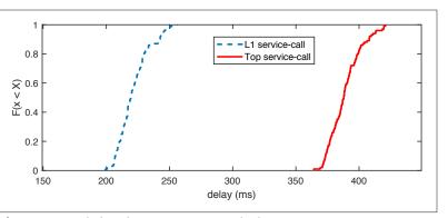
Figure 6. Control plane latency to set-up multi-domain connectivity service.
