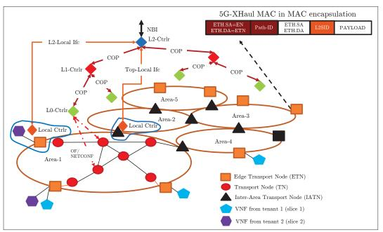
Figure 2. 5G-XHaul control plane architecture.
